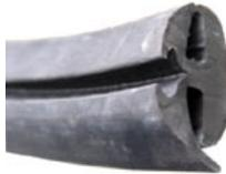
Profilgummi Heckscheibe Limousine (W353 / W1.3)
